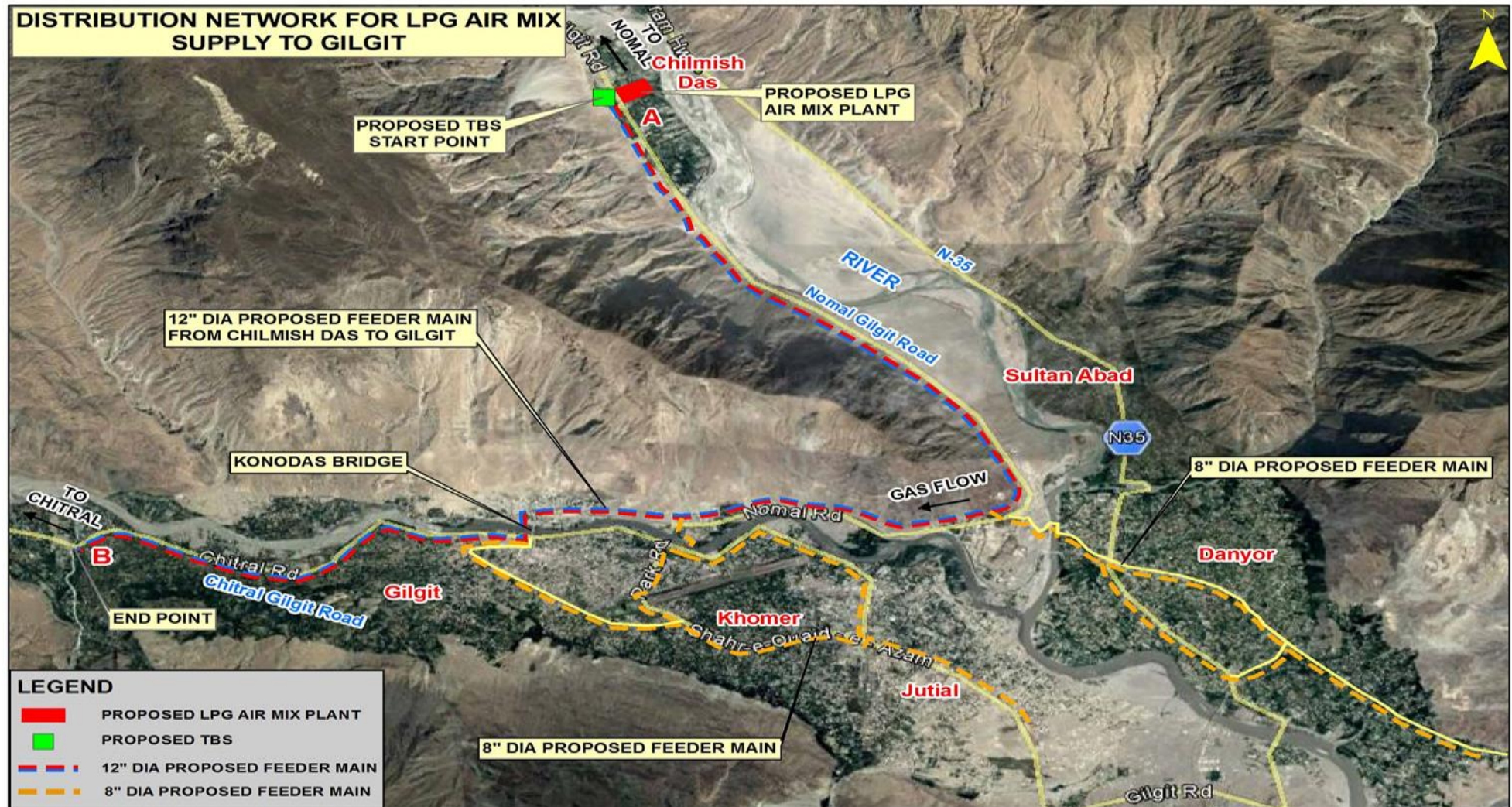
Figure 5: Distribution Network of LPG-Air Mix Plant
