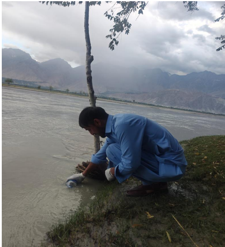
Photograph 7.8 (a): Collection of a water sample from the Indus River, at a representative location away from the project site, for baseline water-quality analysis.
