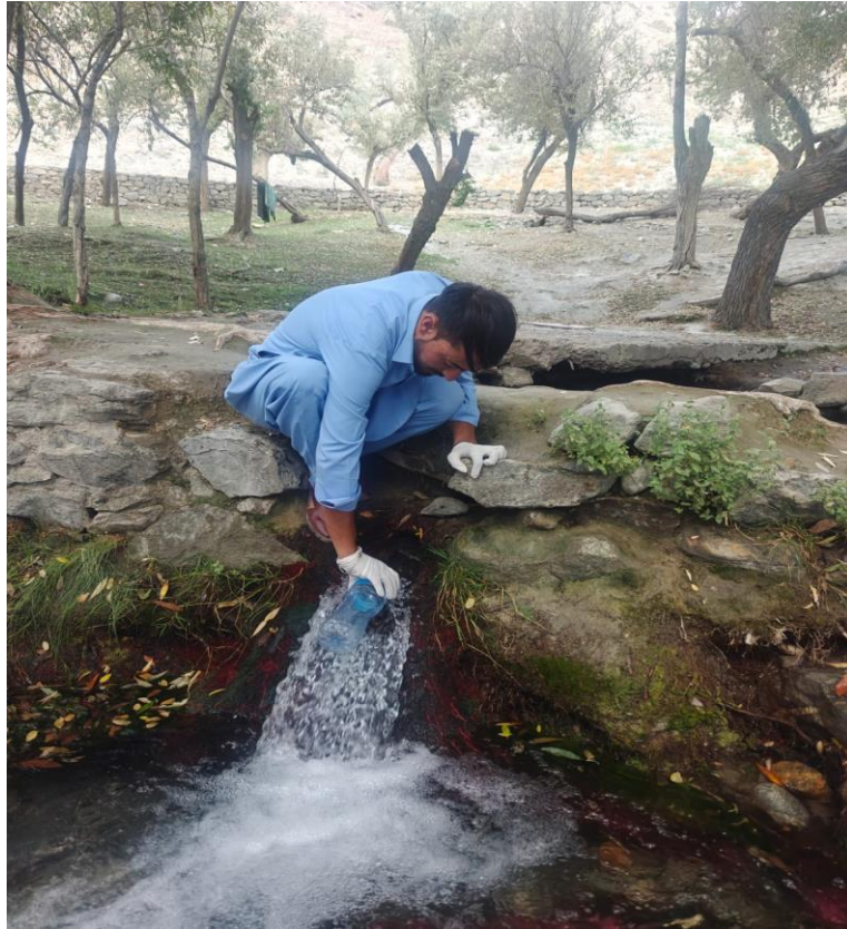
Photograph 7.7: Collection of a water sample from a spring in the vicinity of the project site for baseline water-quality analysis.
