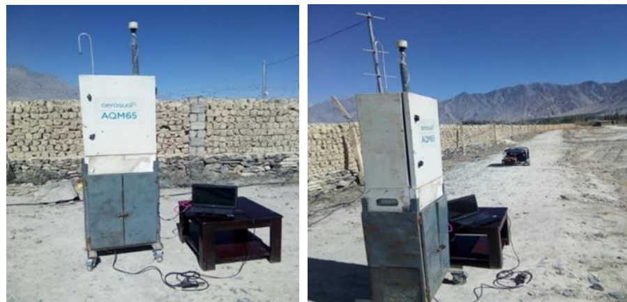
Figure 18: Air Quality Monitoring at Gamba Skardu using AQM65
