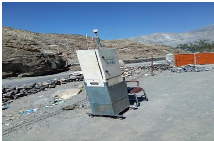
Figure 22: Air Quality Monitoring at Dambudaas using AQM65
