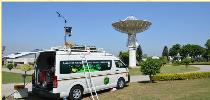
Figure 3.8: SUPARCO Air Monitoring Mobile Laboratory
