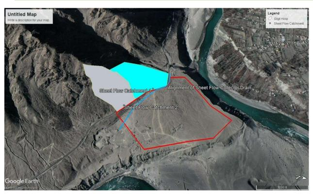
Figure 7 Extents of Sheet Flow Catchments and the proposed alignment of Sheet Flow Collector Drain
