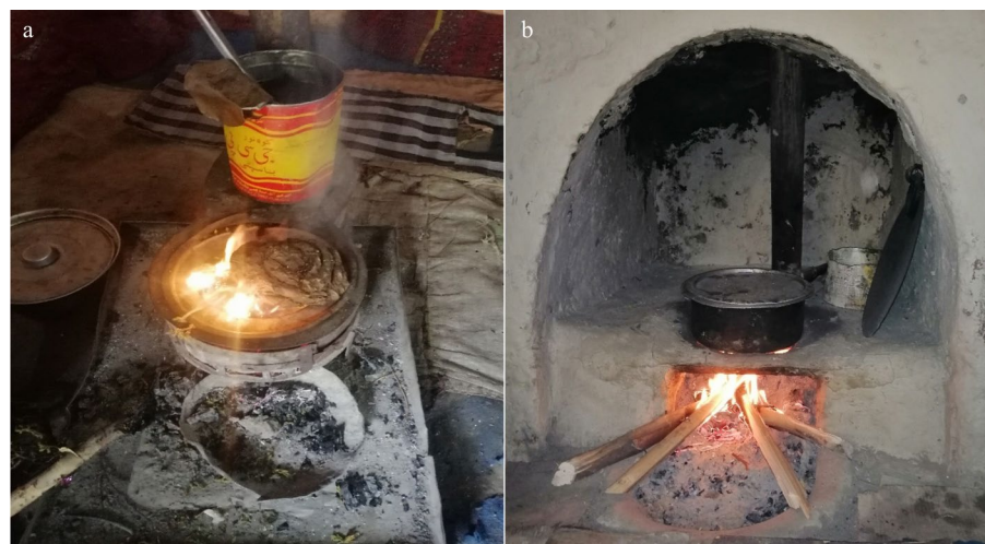
Fig. 10 Traditional stove ( Bukhari ) using animal dung and wood from Hoper, Nagar (a); open-chamber stove using wood from Astore (b)
